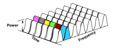
**Traffic** channels: different time slots are allocated to different users, for example, DAMPS and GSM
