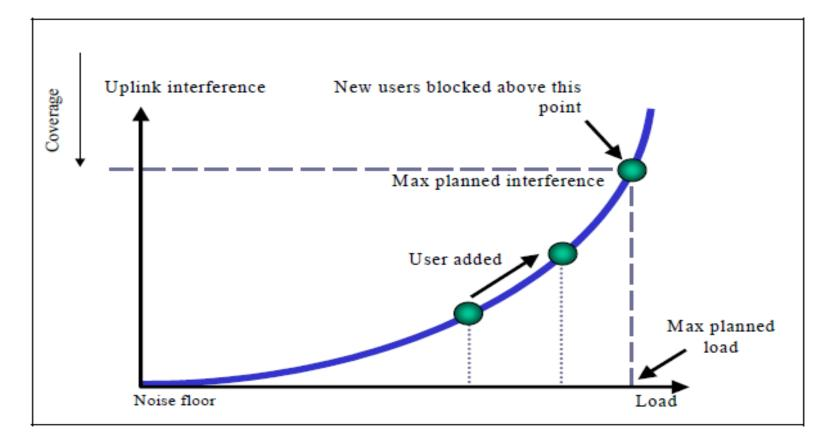
The purpose of Admission Control is to selectively deny access request in order to limit the load, and so avoids excessive triggering of congestion control.
