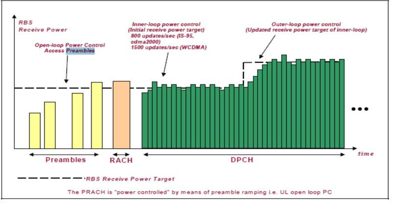
Power control is necessary in any spread spectrum system to ensure that each user transmits and receives just about the right amount of power to maintain the connection quality while at the same time causing as little interference as possible to other users. The output power of the UE is then adjusted at a rate of 1500 times per second.
