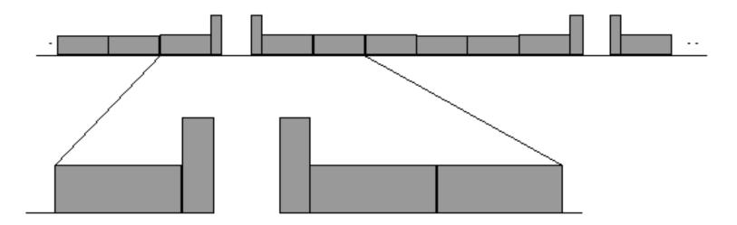
Objective of compressed mode: for UE to realize measurement and synchronization to target cell when inter-frequency handover and inter-system handover is required.
