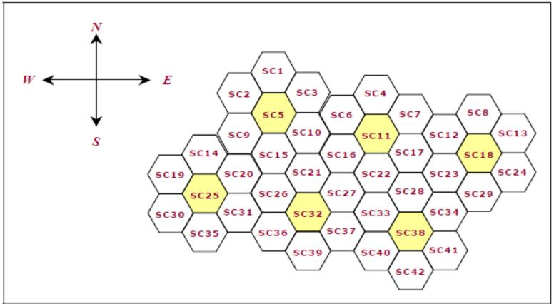
The number of codes used in the downlink is restricted to 8192 in total. 512 of these are primary codes (the rest are secondary codes, 15 codes per primary) divided into 64 code groups each group containing 8 different codes.
